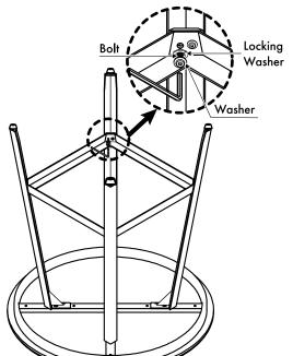
Attach footrest to legs. Loosely screw in one of the bolts to each leg. Repeat with second bolt and tighten All bolts.
