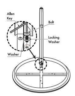
Attach legs loosely to tabletop using the Allen Key.
