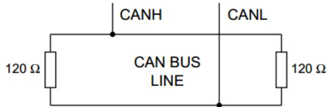
Each end of the CAN bus is terminated with 120Ω resistors in compliance with the standard to minimize signal reflections on the bus.
