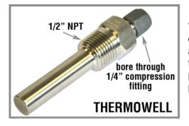
Thermowells are available in 2", 4-1/2", or 7-1/2" lengths for insertion depth and have a ½" NPT process connection. They are supplied with a standard stainless steel compression fitting for securing the thermocouple in the thermowell at the appropriate depth. In low pressure applications the thermocouple can be inserted directly into the process through a standard ½" SS tubing compression fitting.
