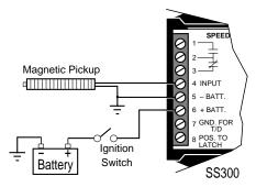
Figure 1: Magnetic Pickup Input
