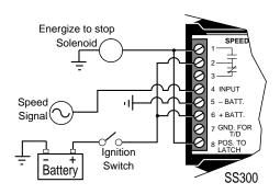
Figure 5: Energize to Stop Solenoid
