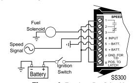
Figure 4: Energize to Run Solenoid
