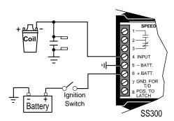
Figure 3: Distributor Ignition Input
