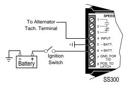
Figure 2: Alternator Tach., Input
