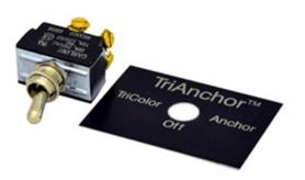
The Weems & Plath OGM Series LX Tri/Color/Anchor Light may be operated using only 2-wires. This Reversing Switch will select between Anchor and TriColor by reversing the polarity of the voltage applied to the two wires. The blue and brown wires from the TriColor/Anchor should be used, and the black ground wire should be cut off and protected from touching the mast or any other metalic objects. This ground wire is not used in 2-wire operation.
