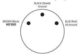
There are three wires in the supplied mating yellow/black cable, however you will only use <u>two</u> wires for the Steaming/Masthead Light (#LX3-MH). The proper connection for these wires is shown in the following diagram:
