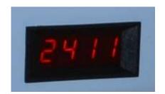
The 4-digit LED display indicates the speed that has been set in rpm. Regulation of the speed takes place continuously by turning the rotary knob in a clockwise direction. (See control panel page 9, control No. 4)
